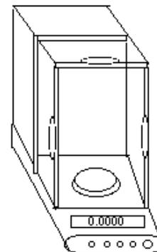
1. Zero the balance by pressing the “TARE” key on the front face. This should give a digital display of either 0.00 g for the top loader and 0.000 g or 0.0000 g for the ones with doors.
